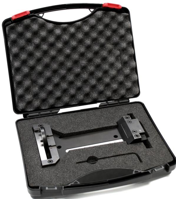
MIRA® can offer an a extension kit for refacing deep seated counterbores on todays truck engines.
