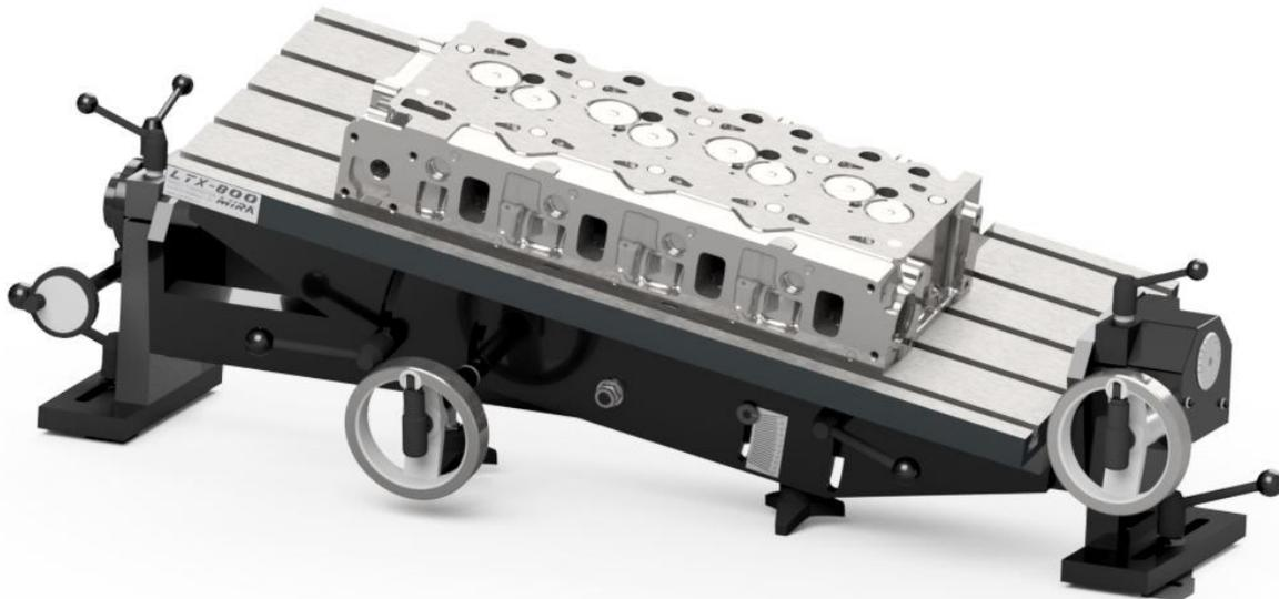
The universal MIRA® leveling table is used for the fast and easy surfacing of cylinderheads, engine blocks, inlet and exhaust collectors and for numerous individual machine shop applications.
