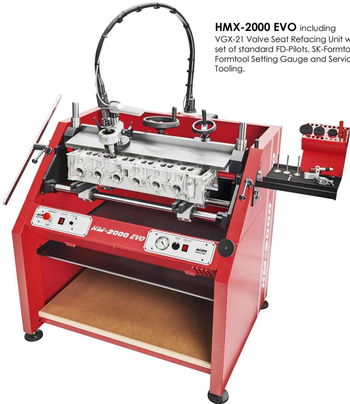
**HMX-2000 EVO** including VGX-21 Valve Seat Refacing Unit with set of standard FD-Pilots, SK-Formtools, Formtool Setting Gauge and Service Tooling.
