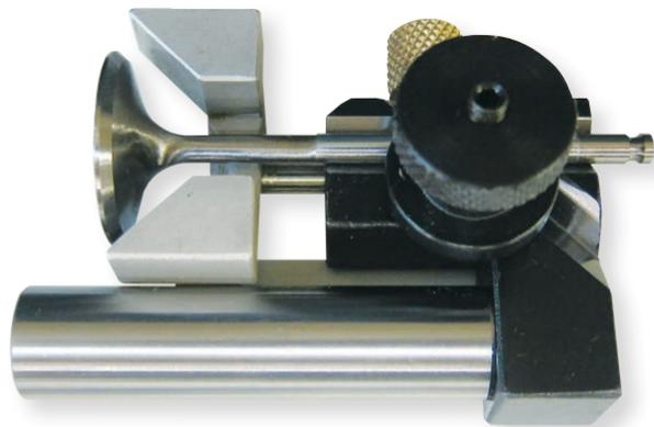
The VR12 has a special device to allow regrinding and chamfering on very short valve stem butt ends.
