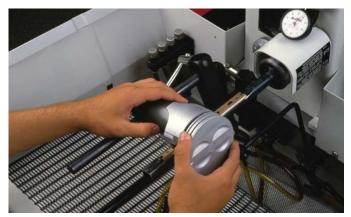
**PISTON PIN BORES** - One of the most critical tolerances in engine rebuilding. Make sure pin holes are perfectly aligned and to size with Sunnen honing. You may even want to "touch up" factory-new piston pin holes to meet your specs.
