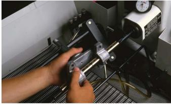
**KING PIN BORES** - Even lower volume operations such as king pin rebuilding can be profitable with the versatile Sunnen LBB-1660.
