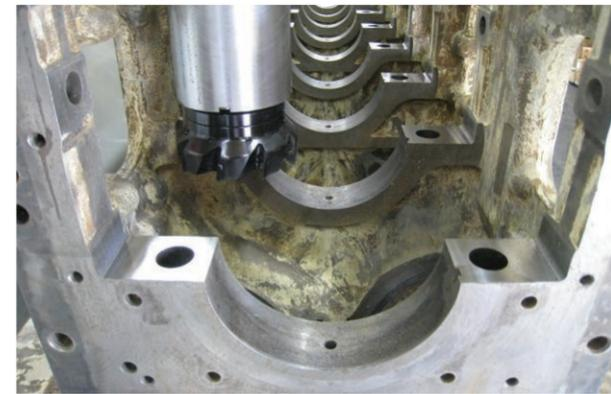
The EM100 series are able to machine main bearing cap registers in the block to ensure they are perfectly flat for maximum contact with main bearing caps. At the same time, the diameter is reduced for line boring back to standard diameter.
