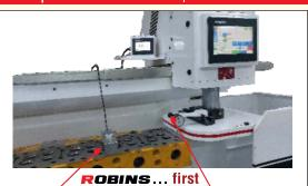
Optional Dual Axis Electronic & Bubble level (use either one) Touch off / levelling dial indicator slides on linear guideways from front to back
